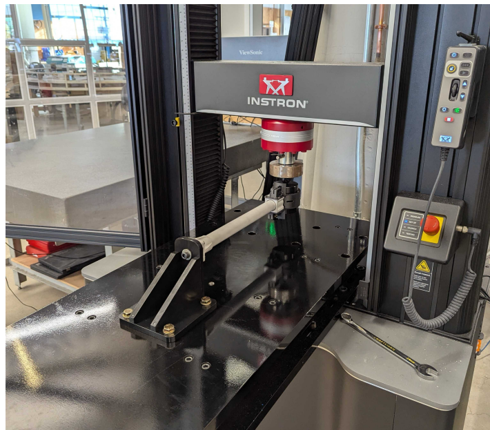
Figure 7: Instron sensor test rig loading setup
