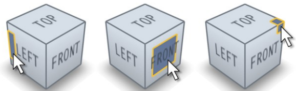
Figure 5. ViewCube Selection Feedback. As the cursor moves over the ViewCube, the piece that would be selected if the user clicked the mouse button is highlighted.
