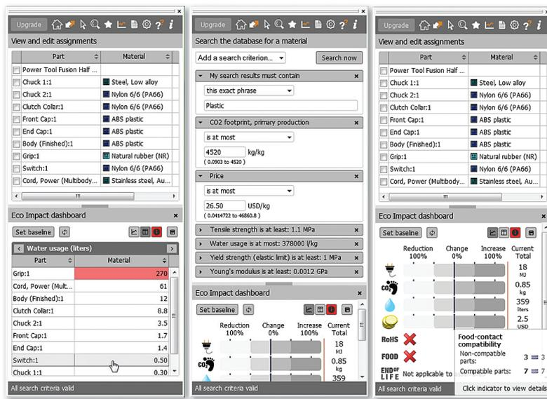
► Figure 2. Eco Materials Adviser: (top left) Material assignments to various parts of the device being designed; (bottom left) Water usage in liters to manufacture the parts; (middle) Materials search interface to help the designer select materials that meet their sustainability, performance, and cost needs; (bottom right) Eco Impact Dashboard showing relative impact from baseline of material changes.
