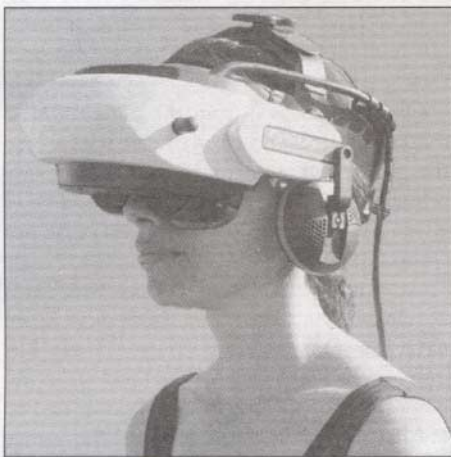
Figure 1: Modern inexpensive HMD: The General Reality CE-200W. (Photo: General Reality Corp.) See page 104 for color image.
