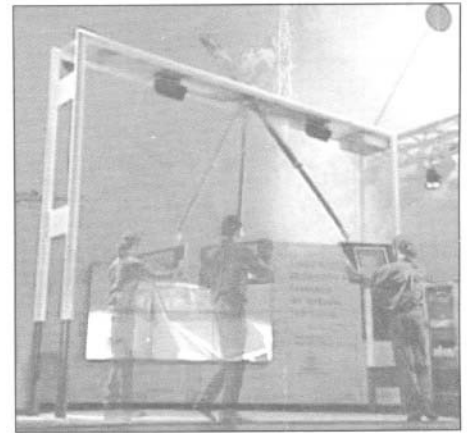
Figure 10: Art+Com virtual car display. This system is essentially a larger format display version of Chameleon. A counter-balanced boom constrains the display movement as well as supports its weight. (Photo: Art+Com). See page 105 for color image.
