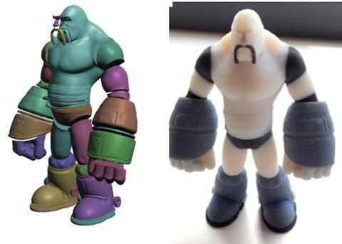
**Figure 1:** Left: exploded view of a non-manifold 3D model created with our system. Right: physical object fabricated with a multi-material 3D printer. White regions are hard solid plastic, and black regions are a flexible, rubber-like material.
