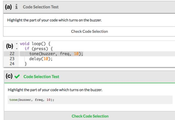
Figure 8. A Code Selection Test. (a) The user is prompted to highlight a section of code; (b) The user highlights the code in the editor; (c) The code is displayed in the test pane and the user clicks to check their response.
