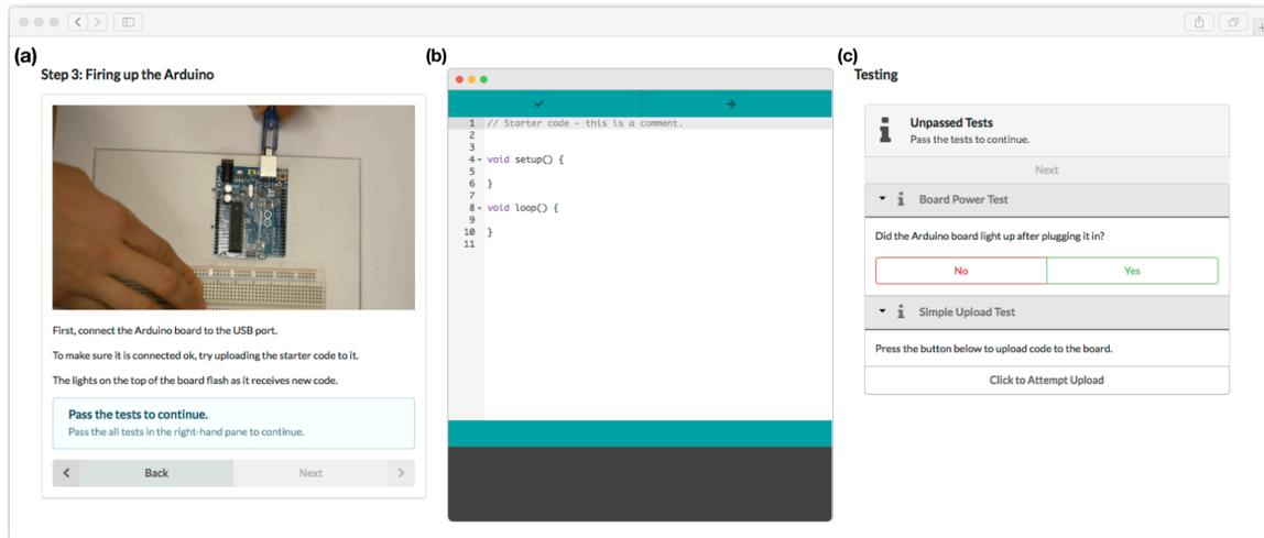
Figure 1: The ElectroTutor interface. The system provides step-by-step tutorials (a) for physical computing projects, a code editing panel (b) and integrated tests used to verify that each step was completed successfully (c).
