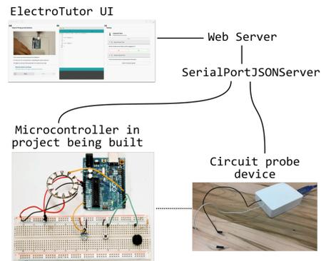
**Figure 12. ElectroTutor system architecture.**
