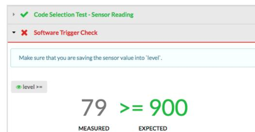
Figure 4. A step with two tests. The first test is collapsed, with a green check mark indicating it has passed. An 'X' icon indicates the second test has failed, and a custom error message is displayed.
