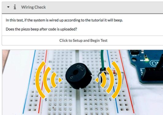
**Figure 10. The Auto-Upload test uses pre-authored code to validate hardware components of the project.**
