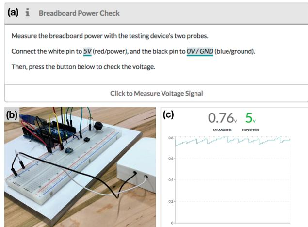
Figure 9. For a voltage test, (a) the user is prompted to attach the circuit probe device to the circuit (b), and run the test. (c) Measurements are then displayed, and the test passes when the expected value is read.
