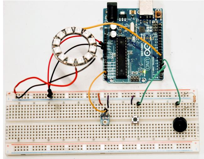
**Figure 13.** The completed Light Sensitive Alarm, consisting of an LED ring, light sensor, buzzer, and a reset button.
