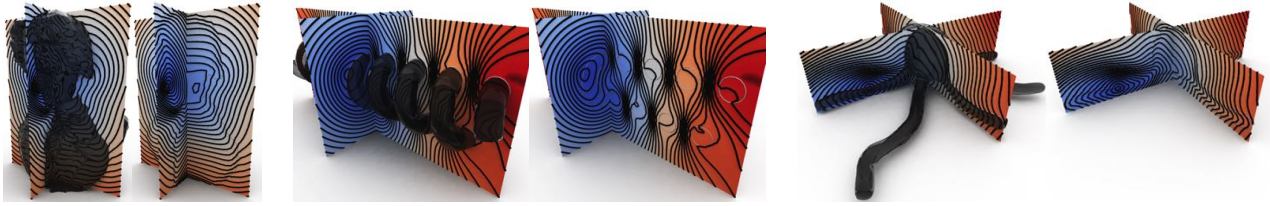
Figure 10: Examples of volumetric distances. The left image in each pair shows a surface (Beethoven bust, spiral, octopus resp.) cut by two planes; the right image shows the volumetric distance function on the two planes.
