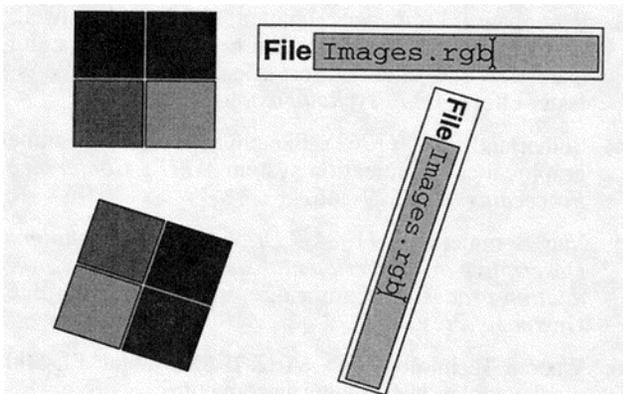
Figure 10. Some widgets are rotation insensitive while others are not. The color palletet on the left is still usable despite the severe rotation. The file name text prompt on the right however becomes very difficult to use at the similar rotation.
