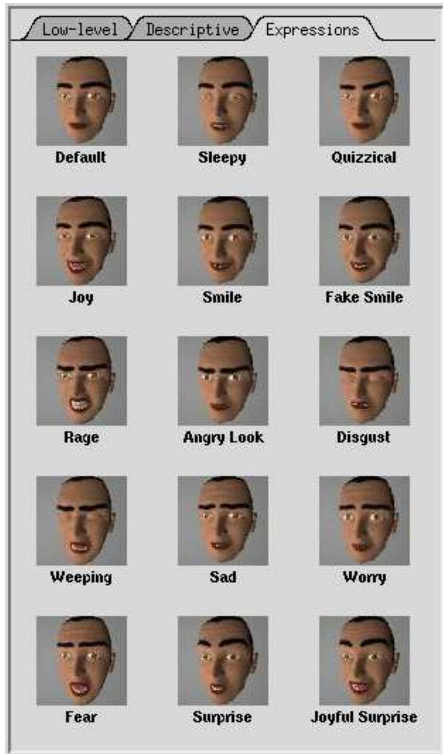
Figure 6.17: The Expressions tab in the animation interface. For each expression, the icon and text provide a button which sets the parameters of the rig to the appropriate values for the expression.
