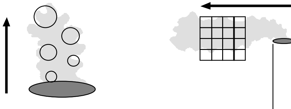
Figure 2: Our simulator computes the evolution of both gases and motion fields. In the picture on the left the disk source generates both gas densities and vortices. The vortices are advected by the single directional heat field. In the picture on the right a turbulence defined on a grid is advected by a directional wind field. In both example, the gas is advected by both fields.
