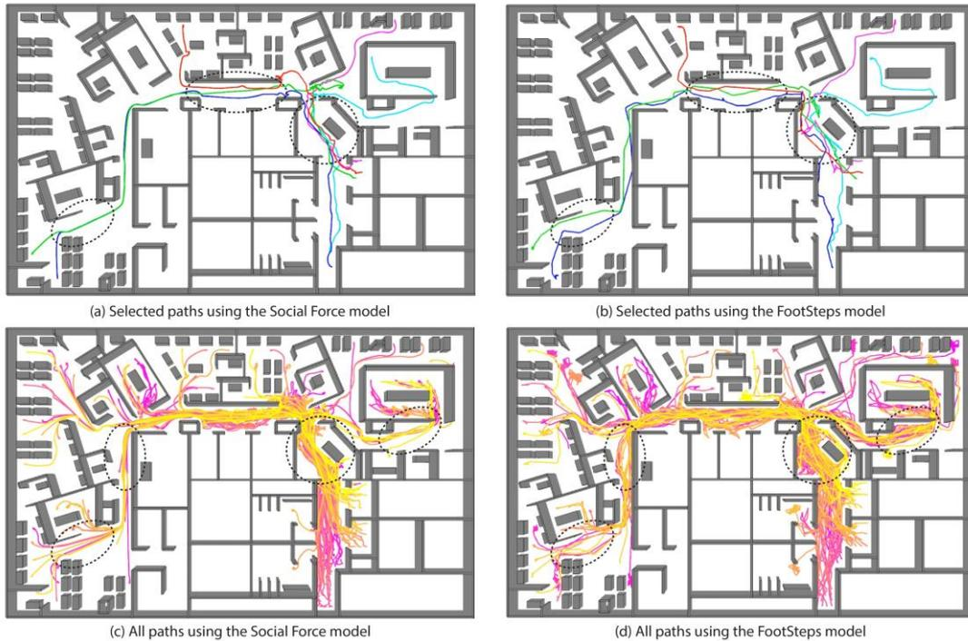
Figure 5: Paths analysis using different occupant movement models
