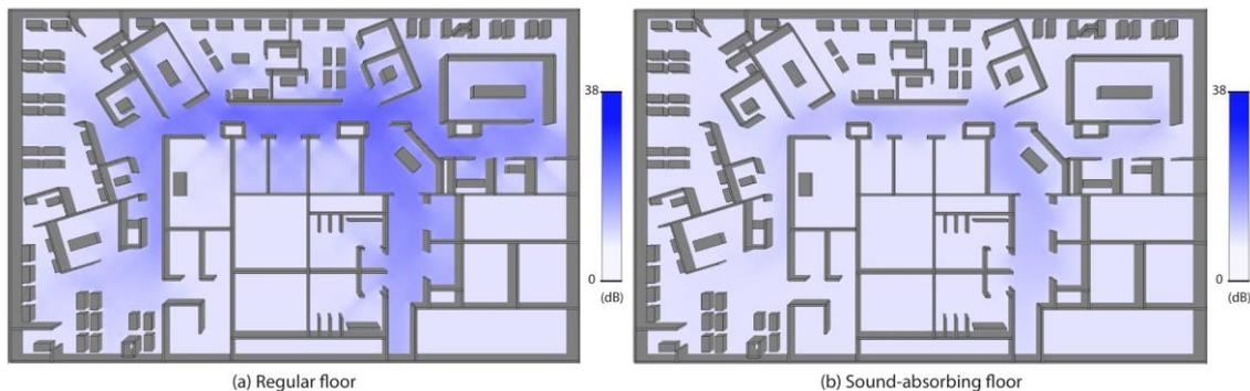
Figure 9: Impact of floor types on sound propagation
