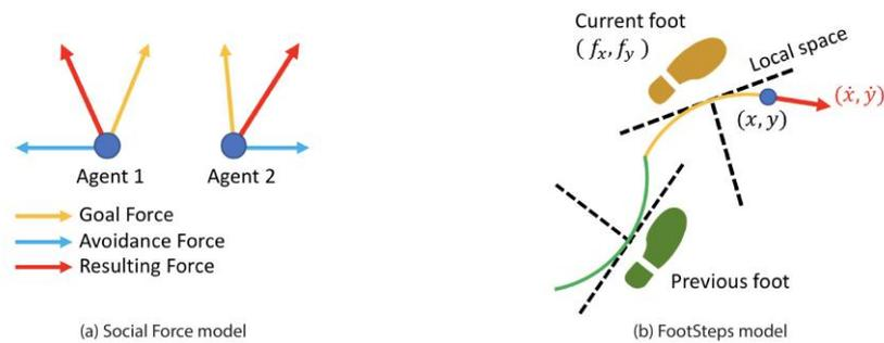
Figure 4: Two established occupant movement simulation models. The Social Force model computes agents' speed and direction as the sum of attractive and repulsive forces. The Footsteps model simulates biped movement using a biomechanically-inspired approach.
