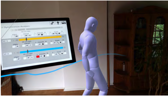
Figure 2: The core components of AvatAR: The virtual humanoid avatar visualizing a person’s detailed posture, a 3D trajectory providing an overview of movement, and the accompanying handheld tablet offering precise control of all visualizations.
