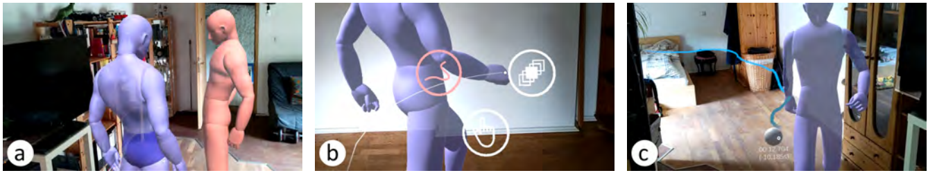
Figure 4: (a) One virtual 3D avatar interacting with the environment with another one walking in the background. (b) Marking menu for the avatar’s hand with the item for trajectories being selected. (c) Trajectory visualizing past and future time frames with the avatar at the center. A handle for adjusting the trajectory’s length is shown as well.
