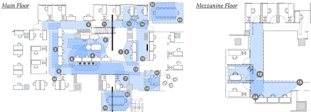
Fig. 3. Office layout used in the study. Grey circles indicate camera positions, and blue regions indicate camera coverage.
